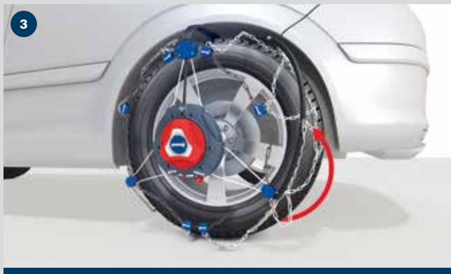
Demounting pewag servomatik
