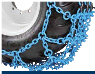
Eg: too loose tensioning in any case
